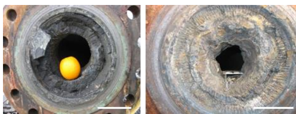
Figure 2. Photographs of scales in surface pipelines downstream of the orifice plate. The scale bar is 10 cm.
